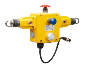
IDEM Z-Range safety switch, cable-pull interlock, 250m maximum pull cable length, emergency stop, dual head, (2) OSSD safety output(s), (1) status monitoring output(s), dual color LED, die-cast aluminum body, 8-pin M12 quick-disconnect.
