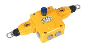
IDEM safety switch, cable-pull interlock, with reset, 250m maximum pull cable length, dual head, (4) N.C. safety output(s), (2) N.O. monitoring output(s), die-cast aluminum body, (4) 1/2in NPT cable entries.
