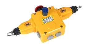
IDEM safety switch, cable-pull interlock, with reset, 250m maximum pull cable length, emergency stop, dual head, (4) N.C. safety output(s), (2) N.O. monitoring output(s), die-cast aluminum body, (4) 1/2in NPT cable entries.
