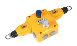
IDEM safety switch, cable-pull interlock, with reset, 250m maximum pull cable length, dual head, (4) N.C. safety output(s), (2) N.O. monitoring output(s), 110 VAC LED, die-cast aluminum body, (4) 1/2in NPT cable entries.
