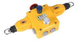
IDEM safety switch, cable-pull interlock, with reset, 250m maximum pull cable length, emergency stop, dual head, (4) N.C. safety output(s), (2) N.O. monitoring output(s), 110 VAC LED, diecast aluminum body, (4) 1/2in NPT cable entries.
