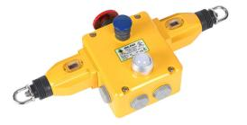
IDEM safety switch, cable-pull interlock, with reset, 250m maximum pull cable length, emergency stop, dual head, (4) N.C. safety output(s), (2) N.O. monitoring output(s), 24 VDC LED, diecast aluminum body, (4) 1/2in NPT cable entries.
