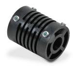
AutomationDirect encoder coupling, 3/8in bore, glass fiber reinforced resin body, setscrew. For use with Koyo TRDA-20 and TRDA-25 series encoders.
