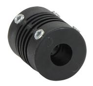
AutomationDirect encoder coupling, 8mm bore, glass fiber reinforced resin body, setscrew. For use with Koyo TRD-N/NA series encoders.
