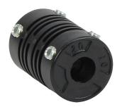
AutomationDirect encoder coupling, 6mm bore, glass fiber reinforced resin body, setscrew. For use with Koyo TRD-S series encoders.
