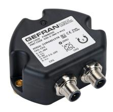
Gefran inclination sensor, 1 axis, +/- 180 degrees, +/-0.5 degrees accuracy, redundant 0-10 VDC output, IP67, thermoplastic (PBT) housing, (2) 5-pin M12 quick-disconnect.
