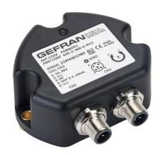
Gefran inclination sensor, 1 axis, +/- 180 degrees, +/-0.5 degrees accuracy, redundant 4-20 mA output, IP67, thermoplastic (PBT) housing, (2) 5-pin M12 quick-disconnect.
