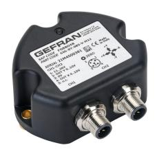
Gefran inclination sensor, 2 axes, +/- 85 degrees, +/-0.5 degrees accuracy, redundant 0-10 VDC output, IP67, thermoplastic (PBT) housing, (2) 5-pin M12 quick-disconnect.
