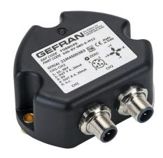
Gefran inclination sensor, 2 axes, +/- 85 degrees, +/-0.5 degrees accuracy, redundant 4-20 mA output, IP67, thermoplastic (PBT) housing, (2) 5-pin M12 quick-disconnect.
