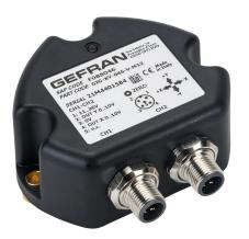
Gefran inclination sensor, 2 axes, +/- 45 degrees, +/-0.5 degrees accuracy, redundant 0-10 VDC output, IP67, thermoplastic (PBT) housing, (2) 5-pin M12 quick-disconnect.
