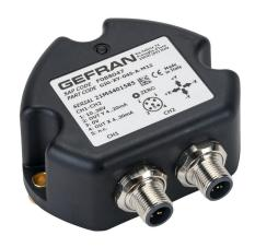
Gefran inclination sensor, 2 axes, +/- 45 degrees, +/-0.5 degrees accuracy, redundant 4-20 mA output, IP67, thermoplastic (PBT) housing, (2) 5-pin M12 quick-disconnect.
