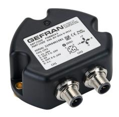
Gefran inclination sensor, 2 axes, +/- 15 degrees, +/-0.5 degrees accuracy, redundant 0-10 VDC output, IP67, thermoplastic (PBT) housing, (2) 5-pin M12 quick-disconnect.
