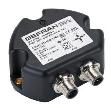
Gefran inclination sensor, 2 axes, +/- 15 degrees, +/-0.5 degrees accuracy, redundant 4-20 mA output, IP67, thermoplastic (PBT) housing, (2) 5-pin M12 quick-disconnect.
