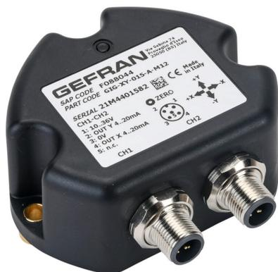
Gefran inclination sensor, 2 axes, +/- 15 degrees, +/-0.5 degrees accuracy, redundant 4-20 mA output, IP67, thermoplastic (PBT) housing, (2) 5-pin M12 quick-disconnect.
