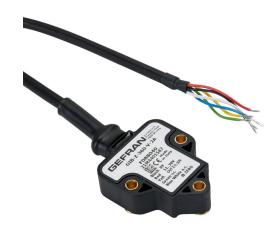
Gefran inclination sensor, 1 axis, +/- 180 degrees, +/-0.5 degrees accuracy, 0-10 VDC output, IP67 IP69K, thermoplastic (PBT) housing, pigtail, 6.5ft/2m cable length.
