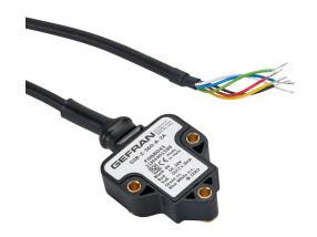
Gefran inclination sensor, 1 axis, +/- 180 degrees, +/-0.5 degrees accuracy, 4-20 mA output, IP67 IP69K, thermoplastic (PBT) housing, pigtail, 6.5ft/2m cable length.
