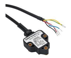
Gefran inclination sensor, 2 axes, +/- 85 degrees, +/-0.5 degrees accuracy, 0-10 VDC output, IP67 IP69K, thermoplastic (PBT) housing, pigtail, 6.5ft/2m cable length.
