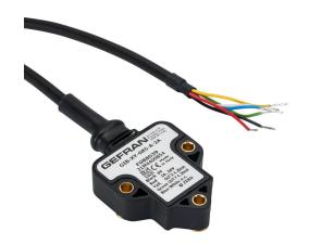
Gefran inclination sensor, 2 axes, +/- 85 degrees, +/-0.5 degrees accuracy, 4-20 mA output, IP67 IP69K, thermoplastic (PBT) housing, pigtail, 6.5ft/2m cable length.
