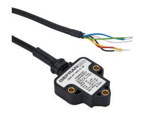
Gefran inclination sensor, 2 axes, +/- 45 degrees, +/-0.5 degrees accuracy, 0-10 VDC output, IP67 IP69K, thermoplastic (PBT) housing, pigtail, 6.5ft/2m cable length.
