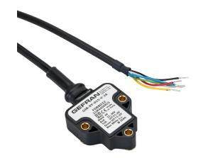
Gefran inclination sensor, 2 axes, +/- 15 degrees, +/-0.5 degrees accuracy, 0-10 VDC output, IP67 IP69K, thermoplastic (PBT) housing, pigtail, 6.5ft/2m cable length.
