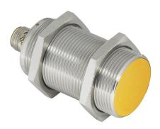
ifm efector inductive proximity sensor, tubular, 30mm diameter x 65mm body, bronze-plated brass housing, PNP, (2) OSSD, >14.5mm enable zone, flush, IP65 IP67 IP68 IP69K, 4-pin M12 quick-disconnect.
