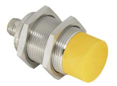
ifm efector inductive proximity sensor, tubular, 30mm diameter x 65mm body, bronze-plated brass housing, PNP, (2) OSSD, >21.5mm enable zone, non-flush, IP65 IP67 IP68 IP69K, 4-pin M12 quick-disconnect.
