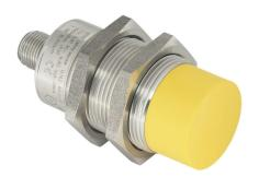
ifm efector inductive proximity sensor, tubular, 30mm diameter x 70mm body, stainless steel housing, PNP, (2) OSSD, 1-15mm enable zone, non-flush, IP65 IP67, 4-pin M12 quick-disconnect.
