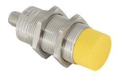
ifm efector inductive proximity sensor, tubular, 30mm diameter x 80mm body, stainless steel housing, PNP, (2) OSSD, 6-12mm enable zone, non-flush, IP68 IP69K, 4-pin M12 quick-disconnect.
