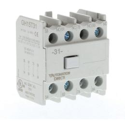
AutomationDirect auxiliary contact, front mount, (3) N.O./(1) N.C. contact(s), 6A @ 120 VAC. For use with all GH15 series contactors.
