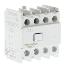
AutomationDirect auxiliary contact, front mount, (1) N.O./(1) N.C. contact(s), 6A @ 120 VAC. For use with all GH15 series contactors.
