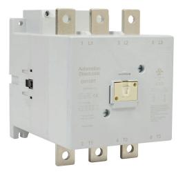
AutomationDirect GH15 series IEC contactor, 210A, (3) N.O. power poles, 120 VAC (60Hz)/110 VAC (50Hz)/110 VDC coil voltage.
