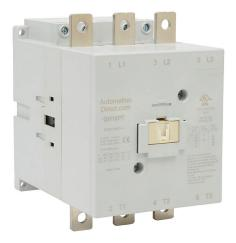
AutomationDirect GH15 series IEC contactor, 175A, (3) N.O. power poles, 120 VAC (60Hz)/110 VAC (50Hz)/110 VDC coil voltage.
