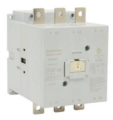
AutomationDirect GH15 series IEC contactor, 150A, (3) N.O. power poles, 120 VAC (60Hz)/110 VAC (50Hz)/110 VDC coil voltage.
