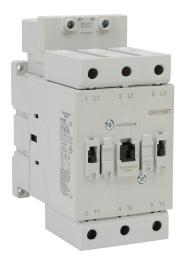
AutomationDirect GH15 series IEC contactor, 110A, (3) N.O. power poles, 240 VAC (60Hz)/220 VAC (50Hz) coil voltage.
