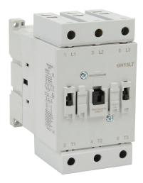
AutomationDirect GH15 series IEC contactor, 95A, (3) N.O. power poles, 240 VAC (60Hz)/212 VAC (50Hz) coil voltage.
