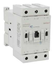
AutomationDirect GH15 series IEC contactor, 95A, (3) N.O. power poles, 120 VAC (60Hz)/110 VAC (50Hz) coil voltage.
