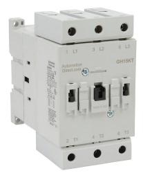
AutomationDirect GH15 series IEC contactor, 80A, (3) N.O. power poles, 120 VAC (60Hz)/110 VAC (50Hz) coil voltage.
