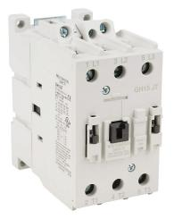
AutomationDirect GH15 series IEC contactor, 63A, (3) N.O. power poles, 120 VAC (60Hz)/110 VAC (50Hz) coil voltage.
