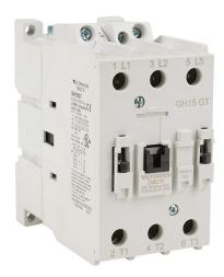
AutomationDirect GH15 series IEC contactor, 40A, (3) N.O. power poles, 120 VAC (60Hz)/110 VAC (50Hz) coil voltage.
