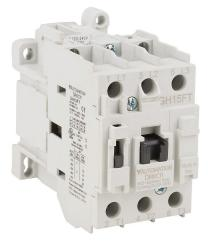
AutomationDirect GH15 series IEC contactor, 32A, (3) N.O. power poles, 240 VAC (60Hz)/220 VAC (50Hz) coil voltage.
