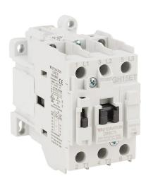
AutomationDirect GH15 series IEC contactor, 25A, (3) N.O. power poles, 120 VAC (60Hz)/110 VAC (50Hz) coil voltage.
