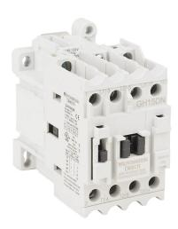
AutomationDirect GH15 series IEC contactor, 16A, (3) N.O. power poles, (1) N.O. auxiliary contacts, 120 VAC (60Hz)/110 VAC (50Hz) coil voltage.
