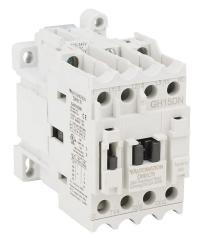
AutomationDirect GH15 series IEC contactor, 16A, (3) N.O. power poles, (1) N.C. auxiliary contacts, 240 VAC (60Hz)/220 VAC (50Hz) coil voltage.
