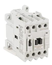
AutomationDirect GH15 series IEC contactor, 16A, (3) N.O. power poles, (1) N.C. auxiliary contacts, 120 VAC (60Hz)/110 VAC (50Hz) coil voltage.
