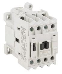
AutomationDirect GH15 series IEC contactor, 12A, (3) N.O. power poles, (1) N.O. auxiliary contacts, 120 VAC (60Hz)/110 VAC (50Hz) coil voltage.
