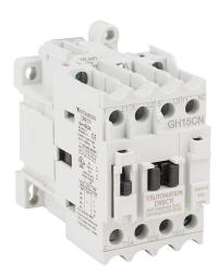
AutomationDirect GH15 series IEC contactor, 12A, (3) N.O. power poles, (1) N.C. auxiliary contacts, 240 VAC (60Hz)/220 VAC (50Hz) coil voltage.
