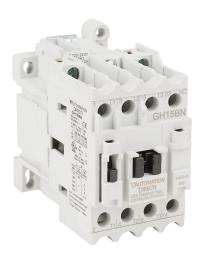
AutomationDirect GH15 series IEC contactor, 9A, (3) N.O. power poles, (1) N.O. auxiliary contacts, 240 VAC (60Hz)/220 VAC (50Hz) coil voltage.
