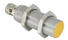
ifm efector inductive proximity sensor, tubular, 18mm diameter x 60mm body, bronze-plated brass housing, PNP, (2) OSSD, >7.5mm enable zone, flush, IP65 IP67 IP68 IP69K, 4-pin M12 quick-disconnect.
