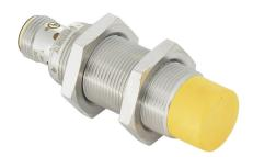
ifm efector inductive proximity sensor, tubular, 18mm diameter x 60mm body, bronze-plated brass housing, PNP, (2) OSSD, >11.5mm enable zone, non-flush, IP65 IP67 IP68 IP69K, 4-pin M12 quick-disconnect.
