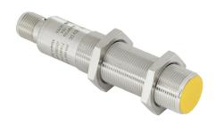
ifm efector inductive proximity sensor, tubular, 18mm diameter x 86.5mm body, bronze-plated brass housing, PNP, (2) OSSD, >10mm enable zone, flush, IP65 IP67, 4-pin M12 quick-disconnect.
