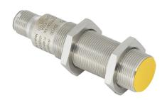
ifm efector inductive proximity sensor, tubular, 18mm diameter x 70.5mm body, bronze-plated brass housing, PNP, (2) OSSD, 1-5mm enable zone, flush, IP65 IP67, 4-pin M12 quick-disconnect.
